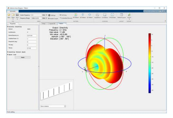
The array has a peak directivity of  ${\bf 11}~{\bf dBi}$  with maximum beam directed at 90 degree azimuth.
