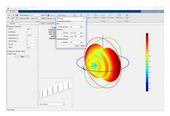
Under **PATTERN** section, click on the **AZ Pattern** and **EL Pattern** to view azimuth and elevation patterns of the linear array. Observe the azimuth and elevation range.
