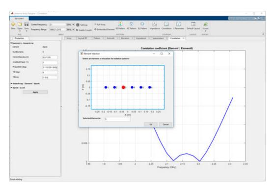
Select element 3 to visualize its 3D radiation pattern. Click  $\mathbf{OK}.$  A new figure named  $\mathbf{Element}\ \mathbf{Pattern}$  is displayed
