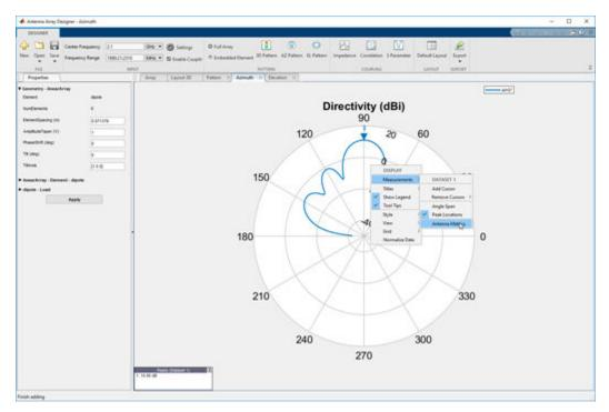
The half-power beamwidth is 18 degree and the sidelobe level is 12.4 dB.
